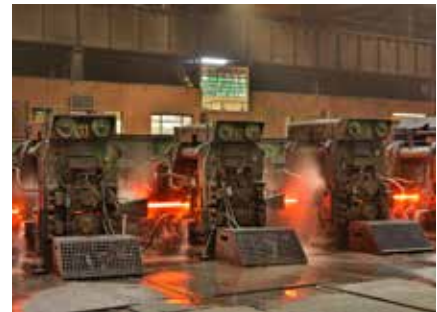
Rod mill – Newcastle Works.
