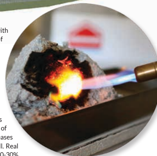
Loose cellulose insulation is very good at filling air pockets, which significantly increases its overall insulation efficiency. Also, in the event of a fire, it performs better than any other commonly used insulation material.
